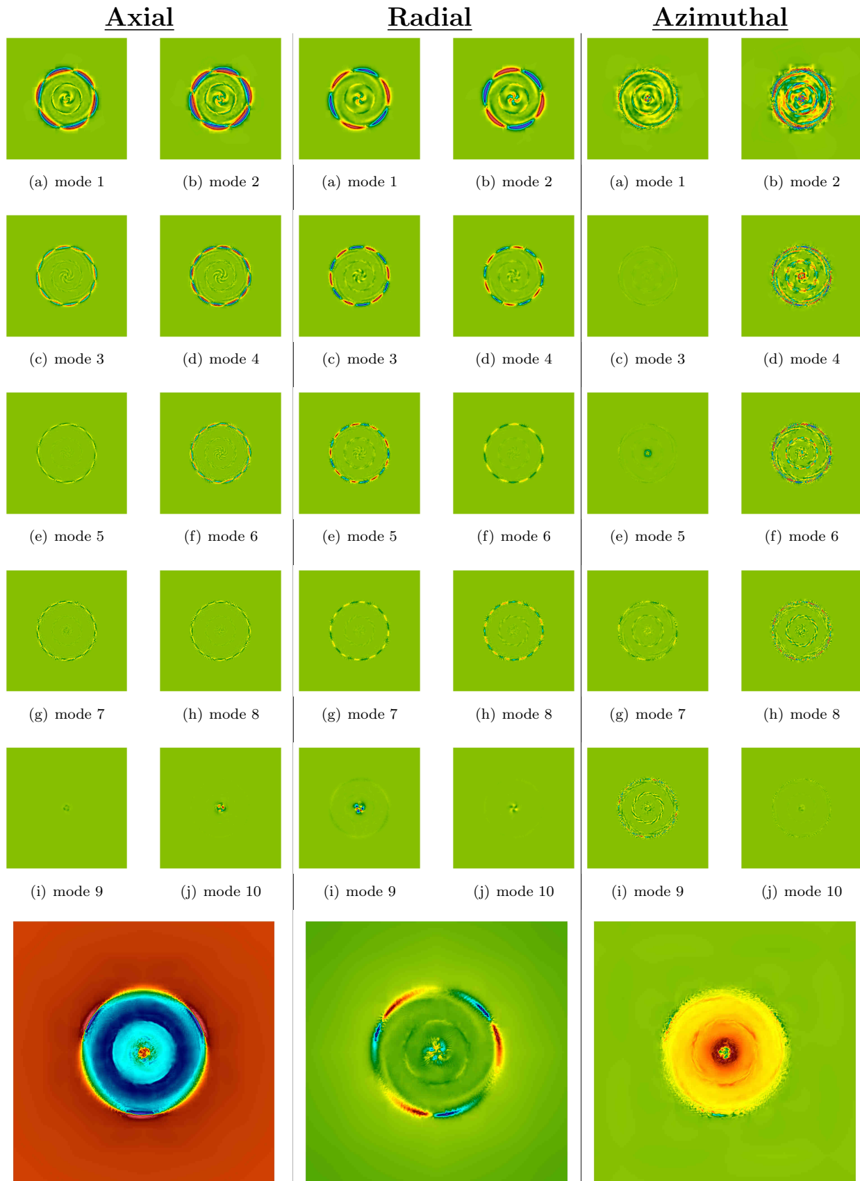
Figure 20. POD modal decomposition and instantaneous flow velocities (bottom) at downstream position x/D = 0.5D .
